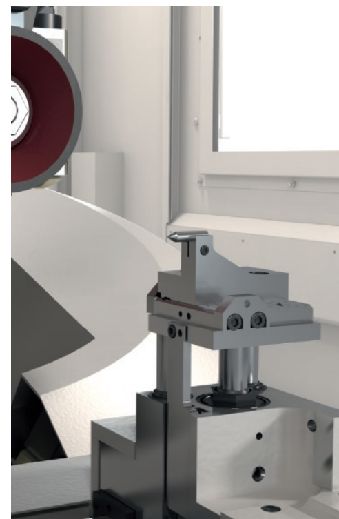
CNC controlled steady rest in different executions
